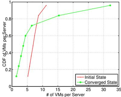
Figure 3: VMs clustering on servers at different states
