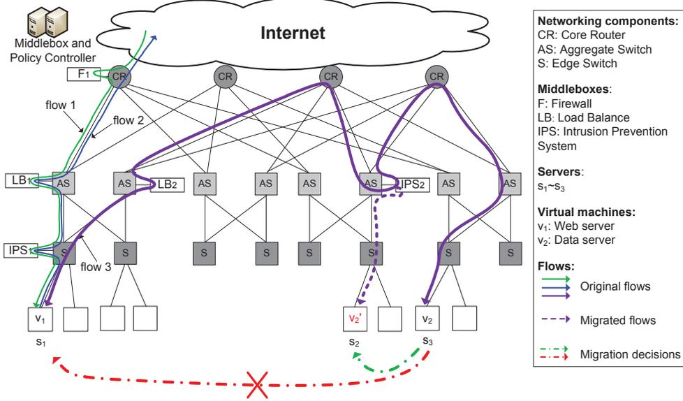
Figure 1: Flows traversing different sequences of middleboxes in DC networks. Without policy-awareness,  $v_2$  will be migrated to  $s_1$ , resulting in longer paths for flow 1 and wasting network resources.
