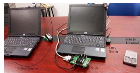
Figure 7. Gateway, video sensor and mobile terminal
